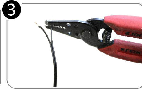
Strip back cable about ¼", identifying polarity. (If using Inspired LED cable, white lettering indicates (+) polarity.)
