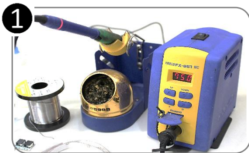
Begin by turning on your soldering iron and allowing it to heat up to at least 700° F.
