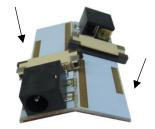
6 Insert flex strip into gap between black sliding latch and beige bridge piece.
