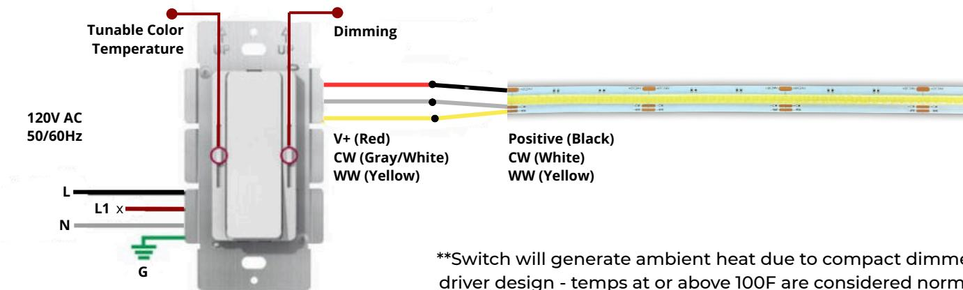
\*\*Switch will generate ambient heat due to compact dimmer/ driver design - temps at or above 100F are considered normal
