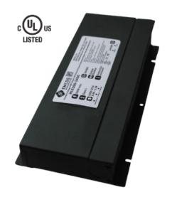
The EMCOD 24V 96W Universal 5-in-1 dimmable driver is designed to accept all different types of dimming. Can be used with Forward Phase, MLV, and Reverse Phase, ELV, TRIAC. Also works with 0-10V dimming (0-10V, 1-10V, Potentiometer) and PWM dimming. Designed to work with Inspired LED's standard 24V LED tape and high density 24V LED and COB tapes.
