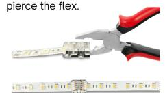
Troubleshooting: If LEDs are flickering, double check connection to be sure flex is fully inserted and secured, if no lights turn on check to be sure polarities are properly matched. Connector must maintain secure contact to avoid overheating.
